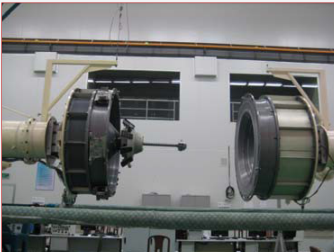
Chinese probe-cone docking mechanism in test (credit: IAF)
